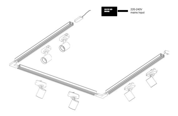
Minimal design low voltage tracklight. Can be installed to track up to the quantity that meets until the total power of central driver connected to single phase track system.
